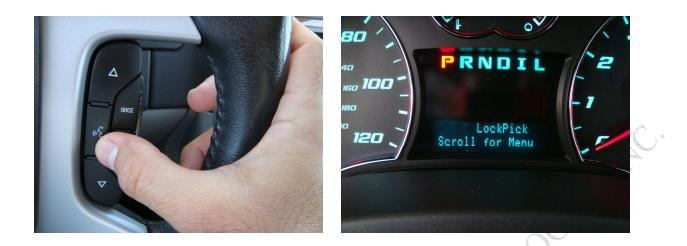
The menus of the Lockpick are controlled using your steering wheel NEXT UP ▲ and NEXT DOWN ▼ buttons to scroll up and down through the Lockpick menus.
