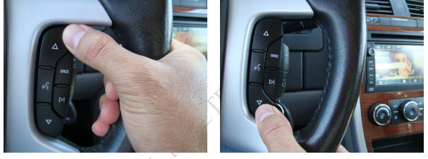
Select any item or option using the SEEK ▶ button. You may also turn off any function without navigating through the text menus by simply pressing the MUTE button 2x.
