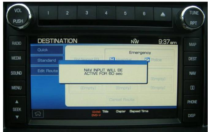
When ENABLE NAV INPUT is selected, the Lockpick will provide 60 seconds for the user to input address information. At the end of 60 seconds it will time out and display NAV INPUT ENDED. You can also end the NAV input override immediately by pressing the PHONE button and holding it for 3 seconds.
