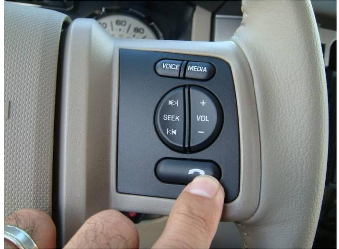
The Lockpick will loop through the functions available with each PHONE button tap. To allow for quick and frequently used menus, it will remember the last function you were on and return to it automatically next time you activate the Lockpick. A sampling of messages and explanations are provided on the next few pages.
