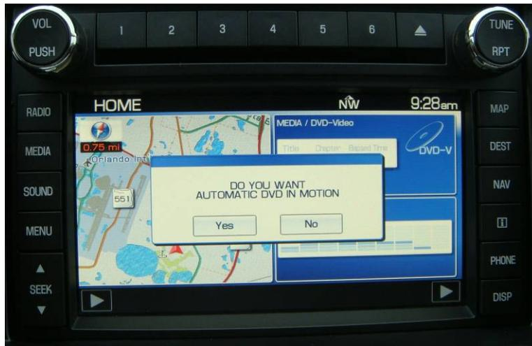
The Lockpick can automatically activate DVD IN MOTION while in Drive gear without any steering wheel or touch screen button presses. If you select NO, the option for viewing DVD IN MOTION will be added to the standard Lockpick menu structure and can be activated manually using the steering wheel and touch screen buttons.
