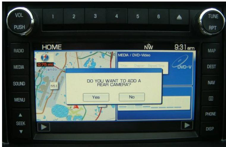
Answering YES to add a rear view camera will set the Lockpick to program the radio for camera operations. After setup, the radio will automatically switch to a camera view while in reverse gear. To make your camera installation simple, there are two optional camera input cables available (depending on your radio type) complete with factory connectors. See installation instructions step 1 for cable applications.
