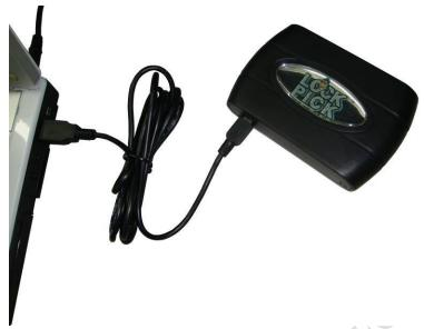
(make sure the module is also connected to the Lockpick harness and vehicle, with the key off)
