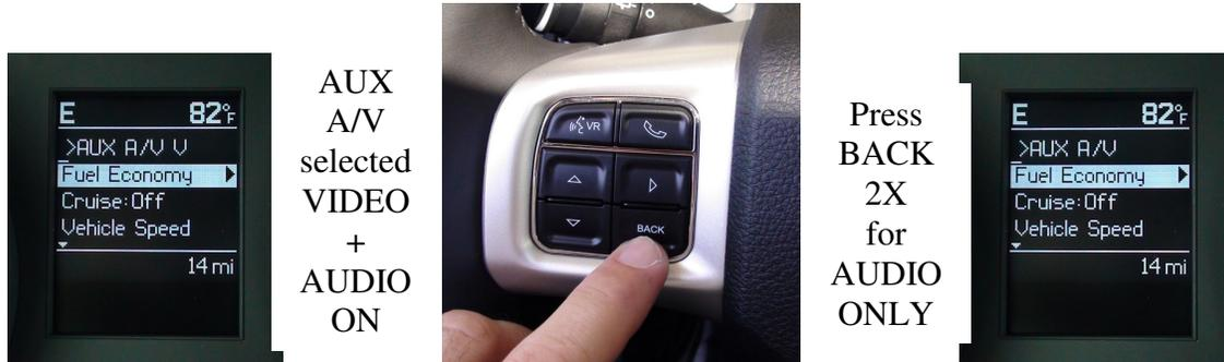
When the AUX A/V function is selected, the Lockpick will enter into a sub menu and display >AUX A/V V. This indicates that the AUX A/V function is now selected (>) and the Video (V) is active and displaying the picture from the source connected to the Video 2 input on the Lockpick module. You may toggle the Video (V) OFF and listen only to the audio by pressing the BACK button on the steering wheel 2x. Press the Back button 2x again and the Video (V) will toggle back ON.
