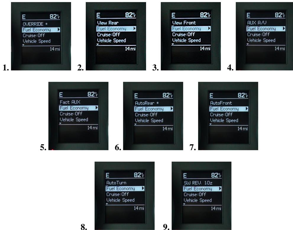
The Lockpick instrument cluster menus will automatically time out after 10 seconds and return you to standard vehicle information or you may press the BACK button 4x again to turn them off immediately. Functions which have been turned on, will indicate with an asterisk next to the selection.
